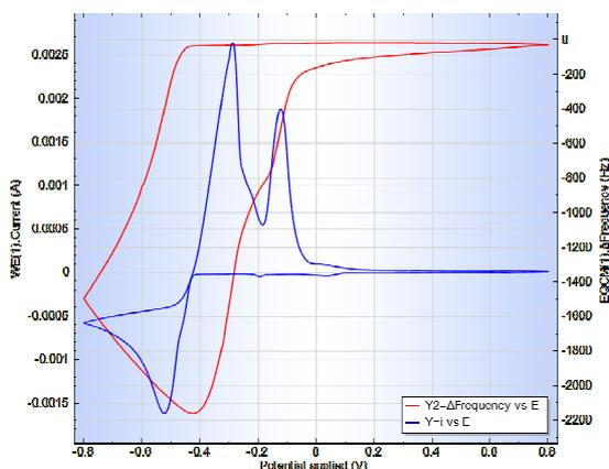
Figure 1 – Cyclic voltammogram (blue curve) and corresponding ΔFrequency change (red curve) for the OPD of lead on gold
