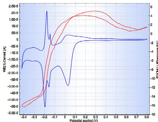
Figure 2 – Cyclic voltammogram (blue curve) and corresponding ΔFrequency change (red curve) for the UPD of lead on gold
