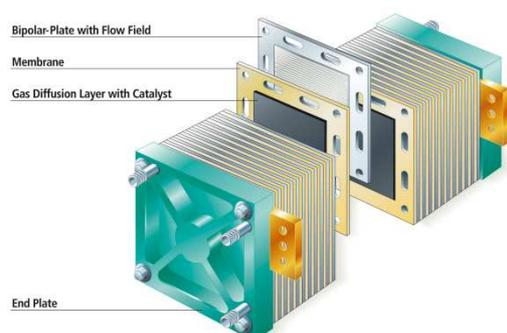
Figure 3 – Schematic overview of a fuel cell stack
