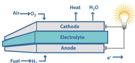
Figure 1 – Working principle of a fuel cell
