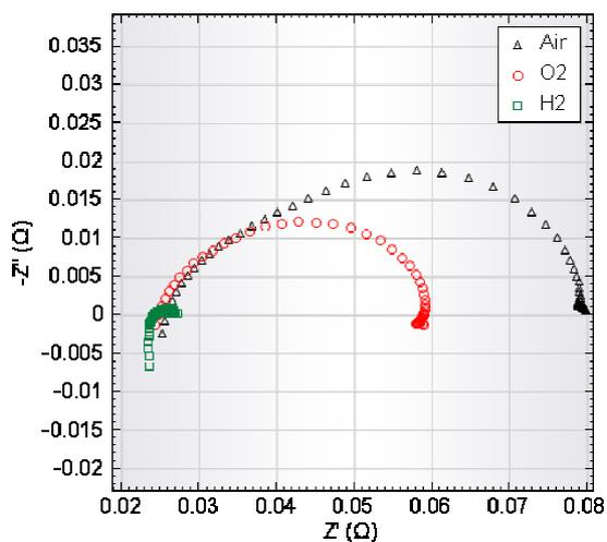
Figure 1 – Results of EIS experiment on a PEM fuel cell with H<sub>2</sub>, O<sub>2</sub> and air at the cathode
